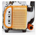
**Pre-separation air filtration system** STIHL long-life air filtration systems with pre-separation achieve perceptibly longer filter life compared with conventional filter systems. Air drawn in is swirled. The larger, heavier particles are ejected. The pre-cleaned air is routed to the air filter via the pre-separator duct.
